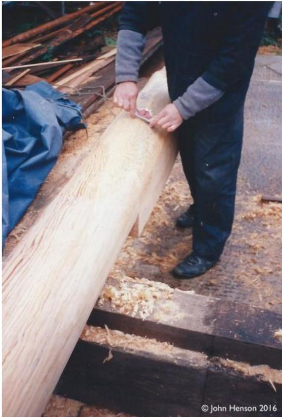
It had taken the best part of six weeks to get to this stage and, it became apparent that there was a massive resin pocket just below the herring hole which would mean that the mast would possibly snap under load.
